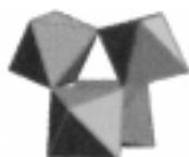
Fig. 2. The basic pyrochlore structural unit: four corner-sharing \text{BO}_6 octahedra.
